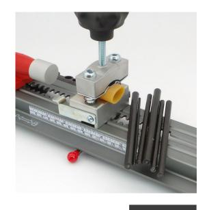
Place the pen inside the cut length of Gripping Tube, and clamp it in the Sliding sled, so that the end that will have the rod inserted, faces the Piston Buffer. If you need more space inside the clamp you can slacken the two hex nuts that hold the clamp in place.
