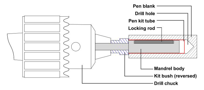
When you have completed turning and finishing, stop the lathe and twist the blank by hand slightly, to allow the blank to come loose and to be removed. It can now be pressed together, not forgetting that you no longer need the finials at either end of the pen, or the clip.
