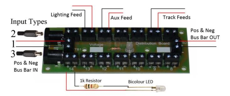
**DCC Connection.** If using it as a DCC Bus Bar you could have up to 18 decoders off the one Distribution Board. The LED will be Orange with DCC power, so will the remote indicator if you use the Bi-coloured LED wired as above.
